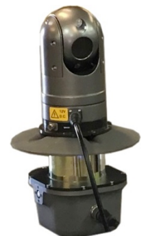
360° laser radar & infrared video surveillance
